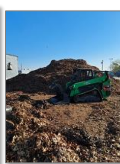
Step 3 CWD utilizes skid steers and other equipment to debag the material, place into transfer ready piles and deliver to the composting facility
